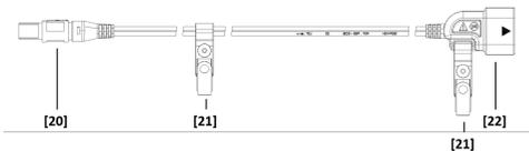
[20] Plug [21] Fixation clips [22] Dongle inlet
