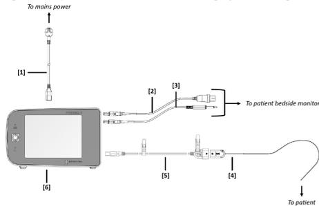
[1] Power cable [2] Pressure cable [3] Temperature cable
