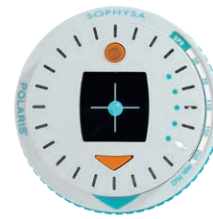
The magnetic center of the valve is found
