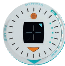
Follow the arrow to find the magnetic center of the valve
